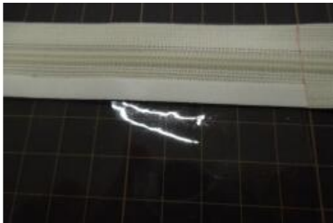
将水溶性两面胶粘带粘在拉链边缘
